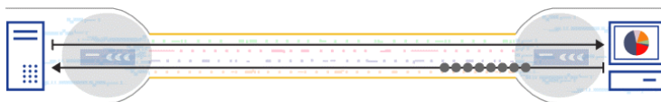
Figure 6. TCP/IP transmission with PFA loads more packets, reduces idle time and overcoming impact of latency
